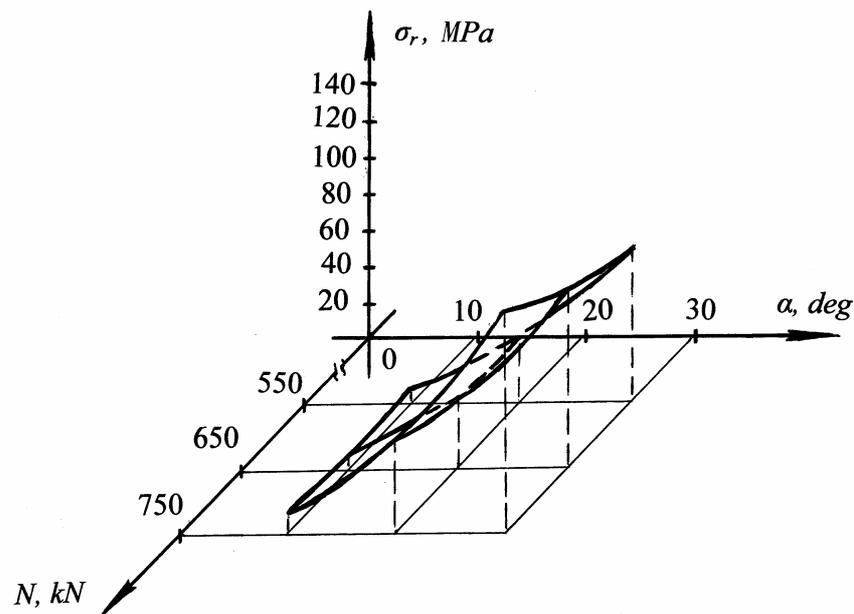
Fig.5 Dependence of the radial  $\sigma_{Gr}$  and tangential  $\sigma_{G\theta}$  stresses acting in the CFCC on the pressure  $p_a$  and angle of steel wire strands twisting  $\alpha$ .
