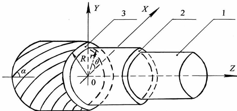
Fig.1. Scheme of hybrid composite cable made of steel, CFCC and GFRP with the cylindrical coordinates system: 1 – CFCC core; 2 – GFRP distributional layer; 3 – steel wire;  $\alpha$  – angle of steel wire strands twisting;  $R$  – radius of the cable;  $Z$ ,  $\theta$ ,  $r$  – cylindrical coordinates;  $X$  – horizontal axis, from which positive direction angle  $\theta$  is counted;  $Y$  – vertical axis.
