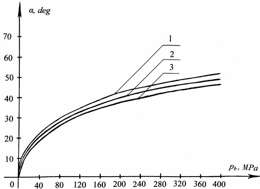
Fig.3 Dependences of pressure  $p_b$  on the angle of steel wire strands twisting  $\alpha$ : 1– dependence, which is obtained at  $N = 750$  kN; 2 – dependence, which is obtained at  $N = 650$  kN; 3 – dependence which is obtained at  $N = 550$  kN.
