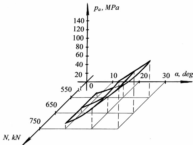
Fig.4 Dependence of pressure  $p_a$  on the axial force  $N$  and angle of steel wire strands twisting  $\alpha$ .
