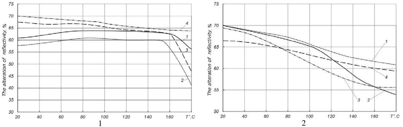
Fig.2 The alteration of reflectivity for  $60^{\circ}$  light dropping angle depending on the temperature:
