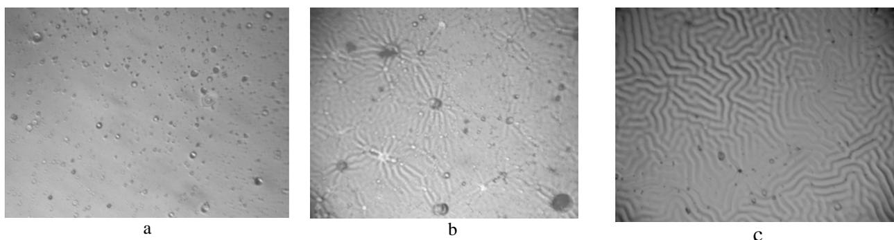
Fig.1 Micro-photos of lacquer coating after tests, x460: a – glossy surface; b - nacre surface; c - lusterless surface
