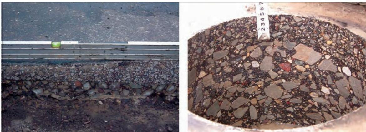
**Fig 2.** Borings made in the pavement structural layer and surfacing (structural layer of pavement: recycled mix ( $h = 2 \times 10$  cm) 50 % additive material, cold mix emulsion AEB-16  $h = 4$  cm)
