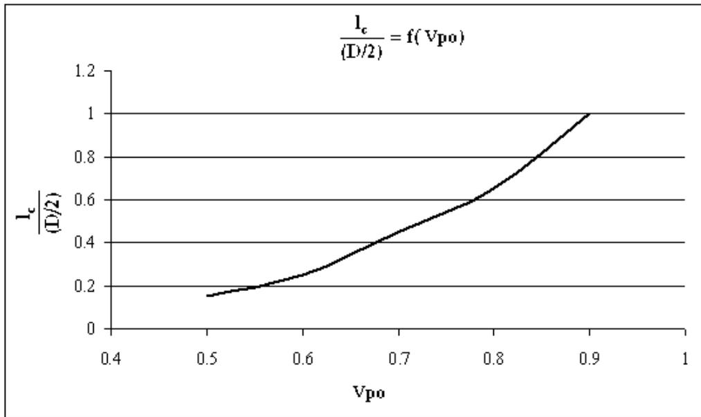
Fig.4. Dependence of relative distance from center for location of substation with maximum efficiency of investments versus absorption probability in center of town
