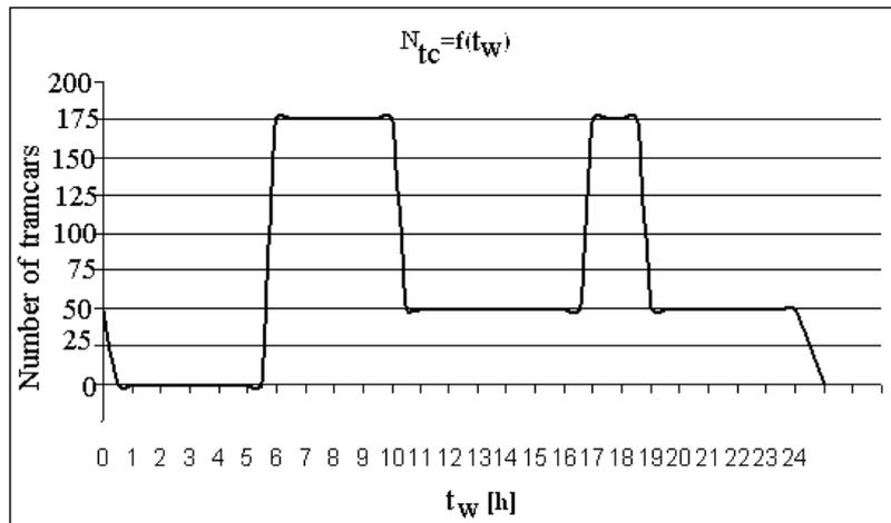
Fig.1. Total number of tramcars in Riga during 24 hours per working day
