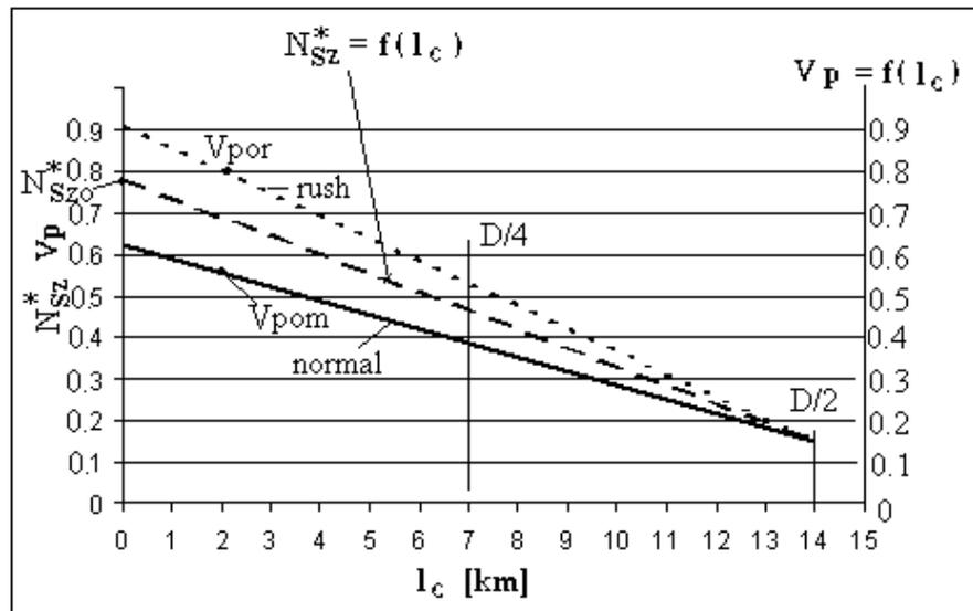
Fig.2. Relative number of tramcars  $N^*_{sz}$  for one radial line and probability  $V_p$  of absorption of recuperated energy in other carriages of the line dependence on distance  $l_c$ ;  $D$  is diameter of town
