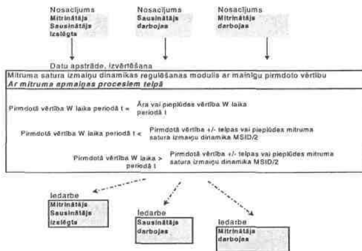
Fig.2-6 The use of the humidity content change dynamics criteria (HCCD) in the regulation scheme.
