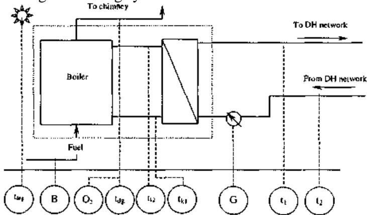
Fig.2.2. CO<sub>2</sub> emission monitoring experimental scheme
