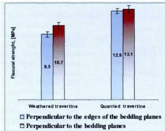
Figure 8. Flexural strength of weathered and quarried Roman travertine perpendicular to the bedding planes.
