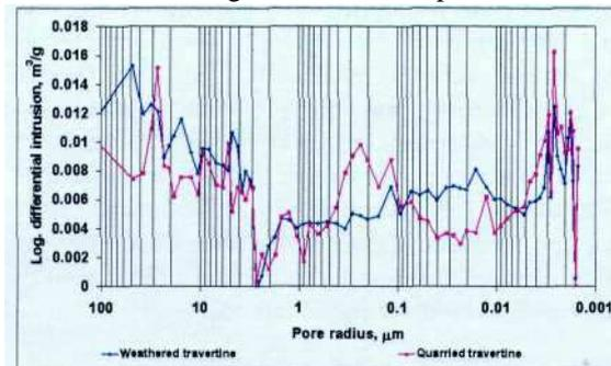
Figure 4. Pore size distribution of quarried and weathered travertine by MIP.
