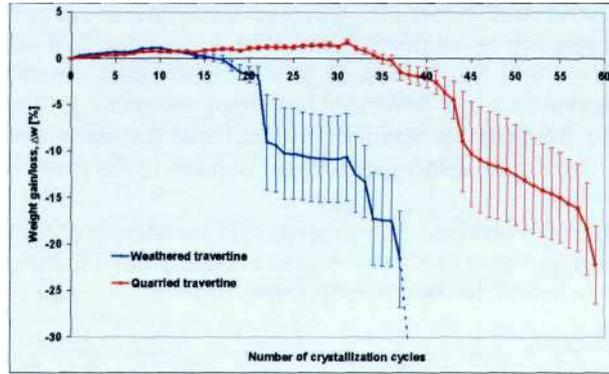
Figure 16. Crystallization test of weathered and quarried Roman travertine.
