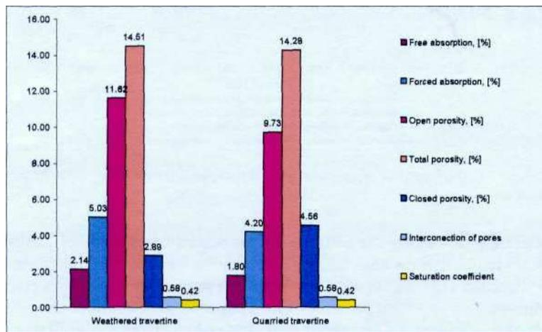
Figure 6. Calculated parameters of physical properties for weathered and quarried Roman travertine.
