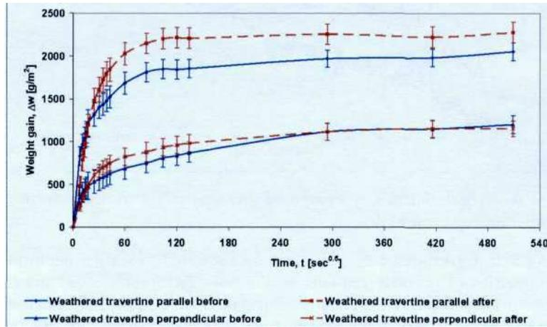
Figure 10. Water absorption by capillarity parallel and perpendicular to the bedding planes of weathered Roman travertine before and after frost test.
