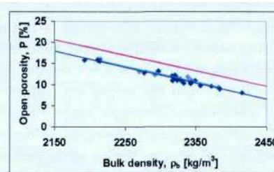
Figure 14. Open porosity versus bulk density for weathered Roman travertine before frost test (deep blue line) and after frost test (light blue line).
