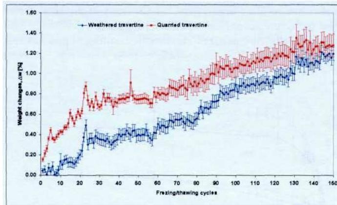
Figure 9. Weight changes of weathered and quarried travertine during freezing/thawing cycles.
