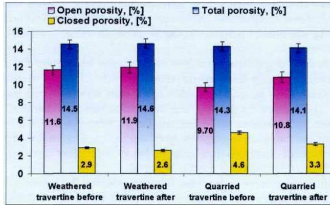
Figure 12. Recalculated values of porosities for weathered and quarried travertine after frost test.
