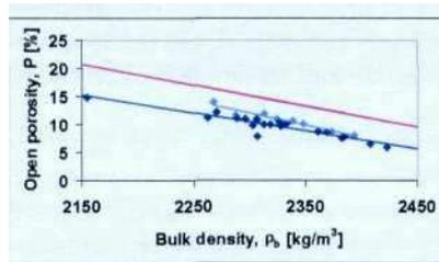
Figure 13. Open porosity versus bulk density for quarried Roman travertine before frost test (deep blue line) and after frost test (light blue line).
