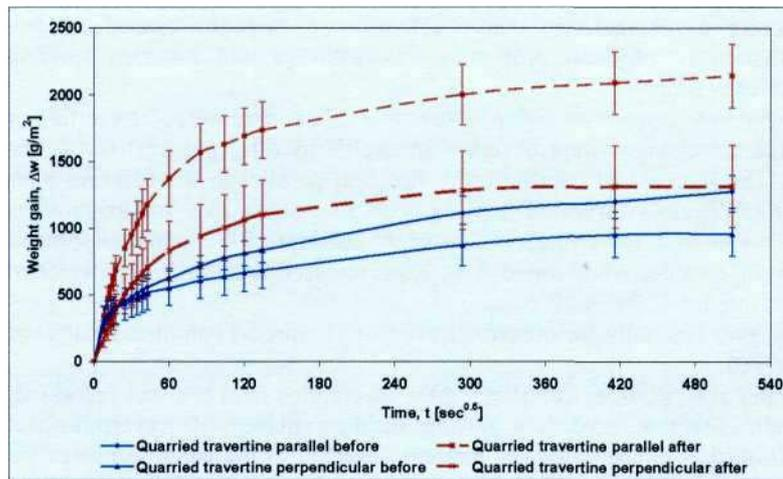
Figure 11. Water absorption by capillarity parallel and perpendicular to the bedding planes of quarried Roman travertine before and after frost test.
