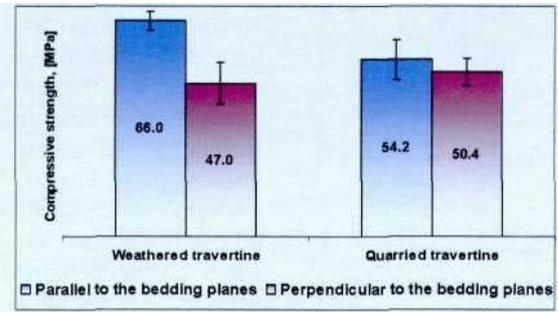
(Figure 7) was done in two directions according to the bedding planes of travertine - with the load applied parallel and perpendicular to the bedding planes. Obtained results of test values for compressive strength have high area of standard errors about 20% due to the high heterogeneity of travertine structure
