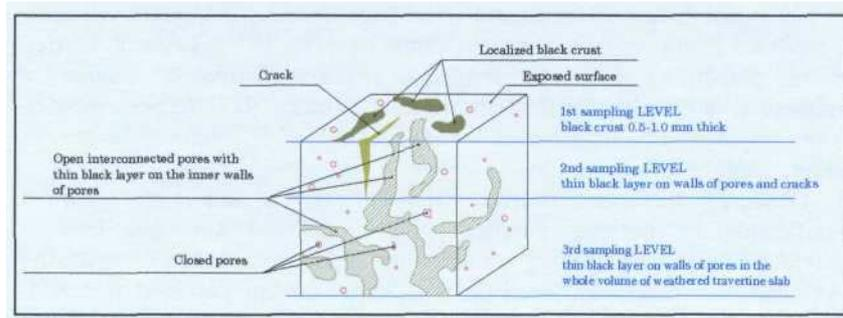
Figure 1. Schematically drawing of sampling levels of deposition layers from weathered Roman travertine from Freedom Monument in Riga.
