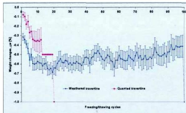
Figure 15. Weight changes of weathered and quarried travertine during freezing/thawing cycles in frosts test by saturation.
