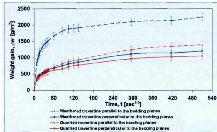
Figure 5. Capillarity of quarried and weathered travertine, weight gain  $[g/m^2]$  vs time  $[sec^{0.5}]$ .
