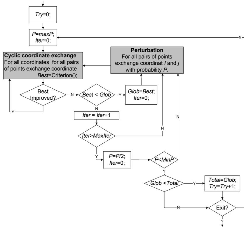
Figure 2. Block diagram of LH optimization algorithm
