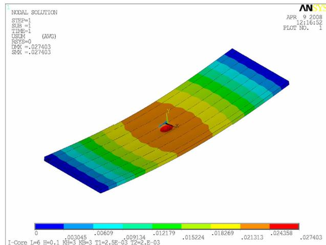
Figure 6. I core sandwich panel deformation
