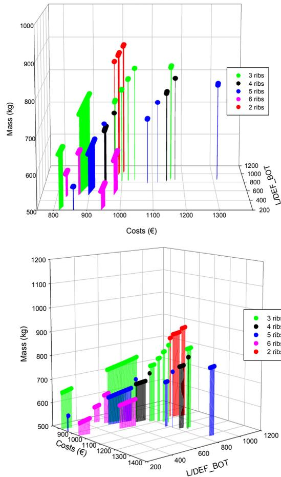
Figure 8. Pareto points for I core sandwich panel
