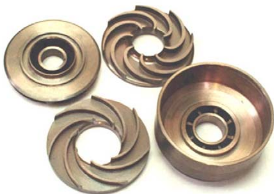
Fig. 5. Components of a centrifugal pump before and after sintering. Diameter of details – 80 mm
