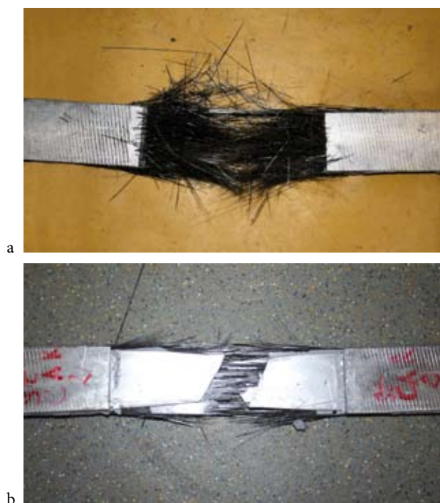
Fig. 3. The types of failure of CFRP and hybrid composite specimens: a – CFRP specimen; b – hybrid composite specimen
