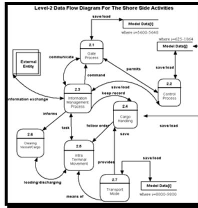
Figure 7 DFD for the Shore Side Processes
