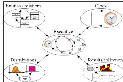
Figure 5 Structure of the Discrete Event Simulation as used by PPS (adapted from Kreutzer, 1986)
