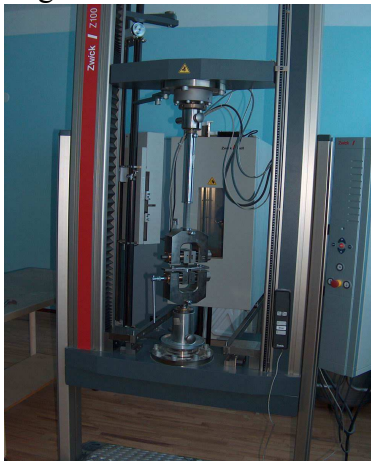
Fig.1 Universal testing system Zwick Z100 with temperature chamber
