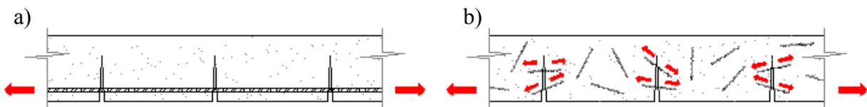
*Fig 1. Post cracking behaviour of: a) traditionally reinforced concrete; b) SFRC*
