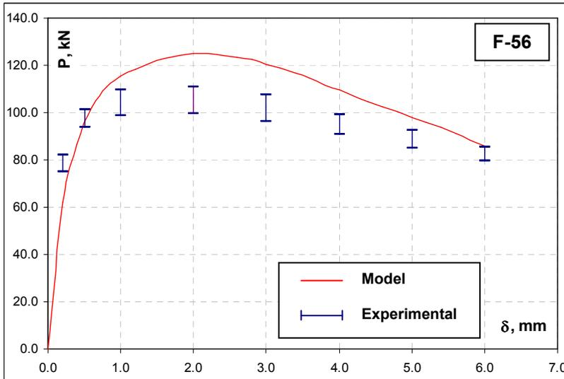
Fig.8. Modelling and experimental bending test results for mix F-56
