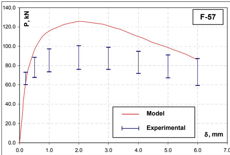
Fig.9. Modelling and experimental bending test results for mix F-57
