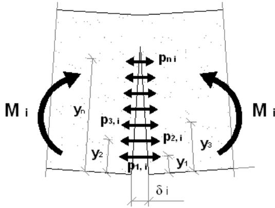
Fig. 7. Scheme of internal forces and moments formed in SFRC beam at post-cracking stage.
