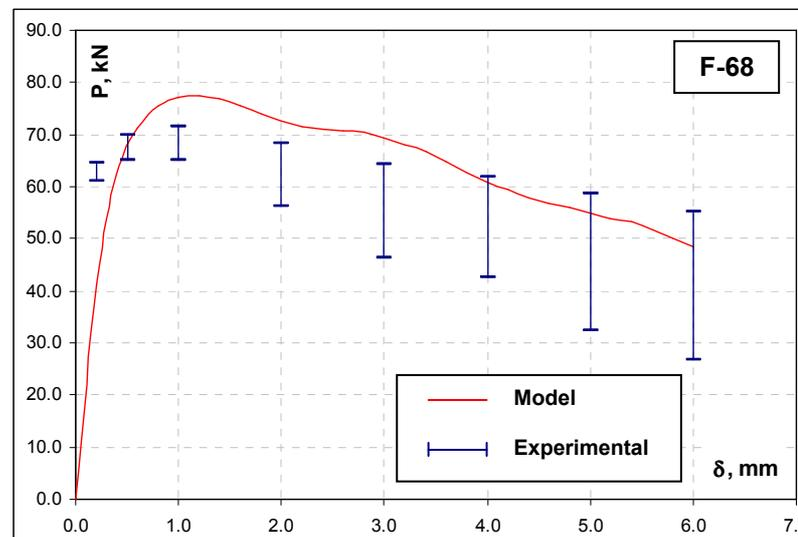
Fig.11. Modelling and experimental bending test results for mix F-68
