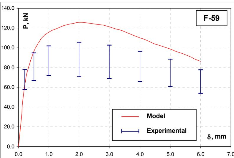
Fig.10. Modelling and experimental bending test results for mix F-59
