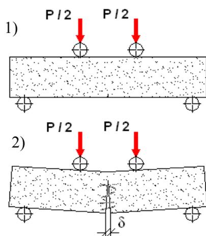
Fig.5. SFRC beam in four point bending test: 1) initial state; 2) post-cracking state
