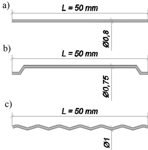
Fig. 2. Steel fibre types: a) straight; b) Dramix fibres; c) Tabix fibres
