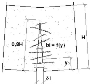
Fig.6. Crack model at beam midpoint
