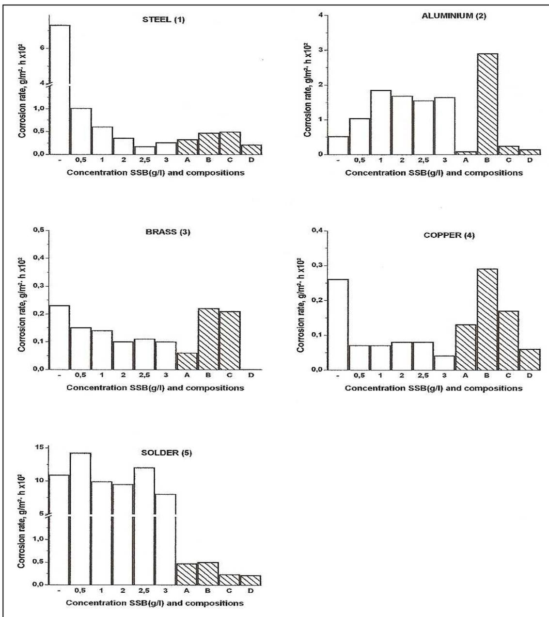
**Fig.5.** Corrosion of steel and non-ferrous metals. Medium ethylene glycol –water (1:1)
