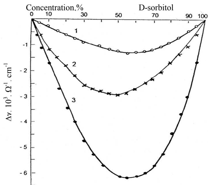
**Fig.3** Deviation from additivity of specific electroconductivity in isomolar series sorbitol- sodium monoborate-water at total concentration 1- 0.25 M; 2-0.5 M; 3-1.0 M
