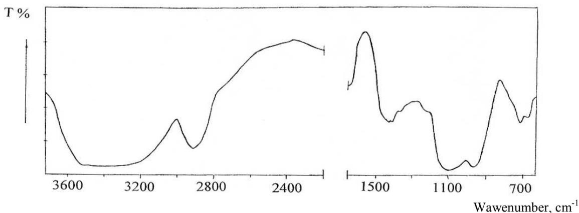
**Fig. 2.** Infrared absorption spectrum of sodium sorbitolborate
