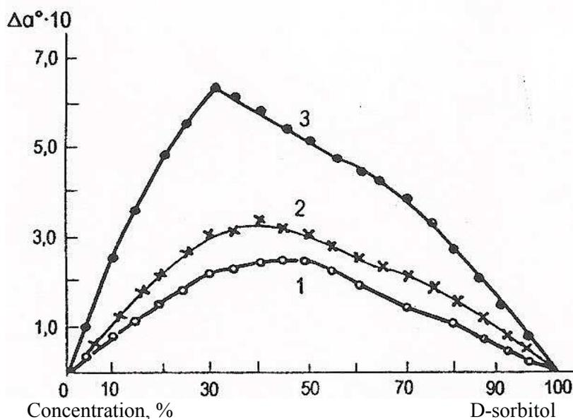
**Fig.4.** Deviation from additivity of rotation angle in isomolar series sorbitol-sodium monoborate-water at total concentration 1- 0.25 M; 2- 0.5 M; 3- 1.0M
