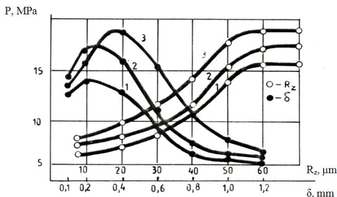
Fig. 3. Dependence of the bonding strength  $P$  on energy of the discharge  $W$ , rod surface roughness  $R_z$  and gap between the details  $\delta$ . Energy levels: 1 –  $W = 6 \text{ kJ/cm}^3$ ; 2 –  $W = 8 \text{ kJ/cm}^3$ ; 3 –  $W = 10 \text{ kJ/cm}^3$  (MIOM equipment with discharge frequency 6 kHz)
