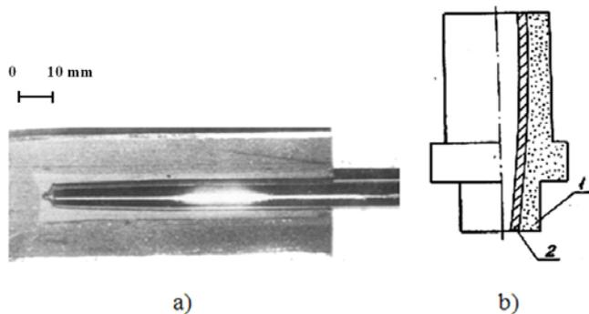
Fig. 2. Multilayer part: a – section; b – scheme; 1 – frame from Fe-Cu powder material; 2 – facing layer from Ni-Co alloy
