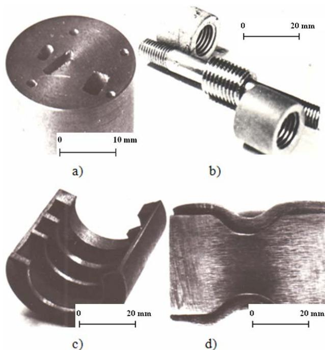
**Fig. 1.** Fe-Cu powder details with complicated shape achieved by MIOM technology
