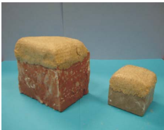
Fig. 5. Sacrificial lime layer on brick and dolomite samples
