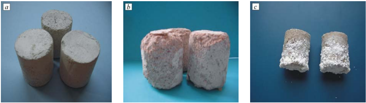
Fig. 2. Lime-based poultice 1 : 2 before exposure (a), after exposure to 0.1 M \text{Na}_2\text{SO}_4 (b), 1 M \text{NaCl} (c) solution for 25 days
