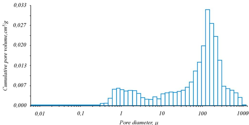
**Fig. 8.** Pore size distribution in the material with the  $\alpha$ - $\text{Al}_2\text{O}_3$  to  $\gamma$ - $\text{Al}_2\text{O}_3$  ratio 1 : 2 after addition of 5 wt% of kaolin and 5 wt% of silica
