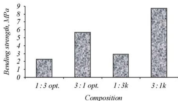
**Fig. 2.** Bending strength. Opt. – Optapix additive; k – kaoline additive
