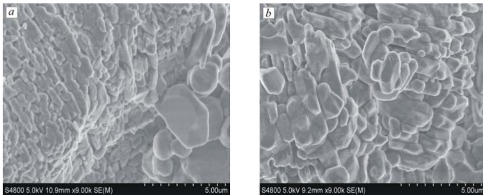
**Fig. 6.** SEM pictures of materials sintered at a temperature of 1600 °C: *a* – with prevalence of coarse-grained  $\gamma\text{-Al}_2\text{O}_3$ ; *b* – with prevalence of fine-grained  $\alpha\text{-Al}_2\text{O}_3$
