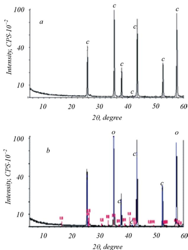
**Fig. 3.** X-ray diffraction of obtained materials: a – with prevalence of coarse-grained  $\gamma$ -Al<sub>2</sub>O<sub>3</sub>; b – with prevalence of fine-grained  $\alpha$ -Al<sub>2</sub>O<sub>3</sub>
