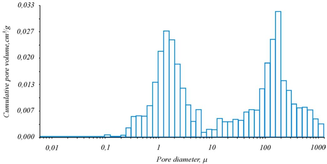
**Fig. 4.** Pore size distribution in the composition with the  $\alpha\text{-Al}_2\text{O}_3$  to  $\gamma\text{-Al}_2\text{O}_3$  ratio 3 : 1 with the prevalence of fine-grained  $\alpha$ -alumina
