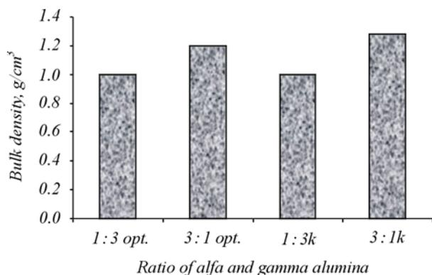
**Fig. 1.** Bulk density of samples. Opt. – Optapix additive; k – kaoline additive
