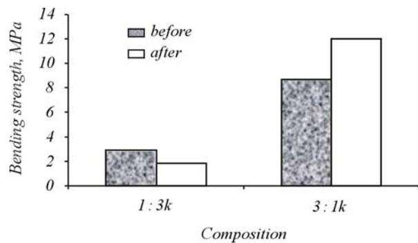
**Fig. 7.** Bending strength of materials with the prevalence of  $\gamma$ - $\text{Al}_2\text{O}_3$  (composition 1 : 3k) and of  $\alpha$ - $\text{Al}_2\text{O}_3$  (composition 3 : 1k) before and after thermal shock testing
