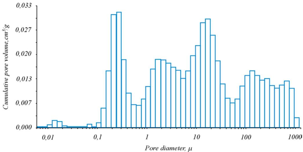
**Fig. 5.** Pore size distribution in a composition with the  $\alpha\text{-Al}_2\text{O}_3$  to  $\gamma\text{-Al}_2\text{O}_3$  ratio 1 : 3k with the prevalence of coarse-grained  $\gamma\text{-Al}_2\text{O}_3$
