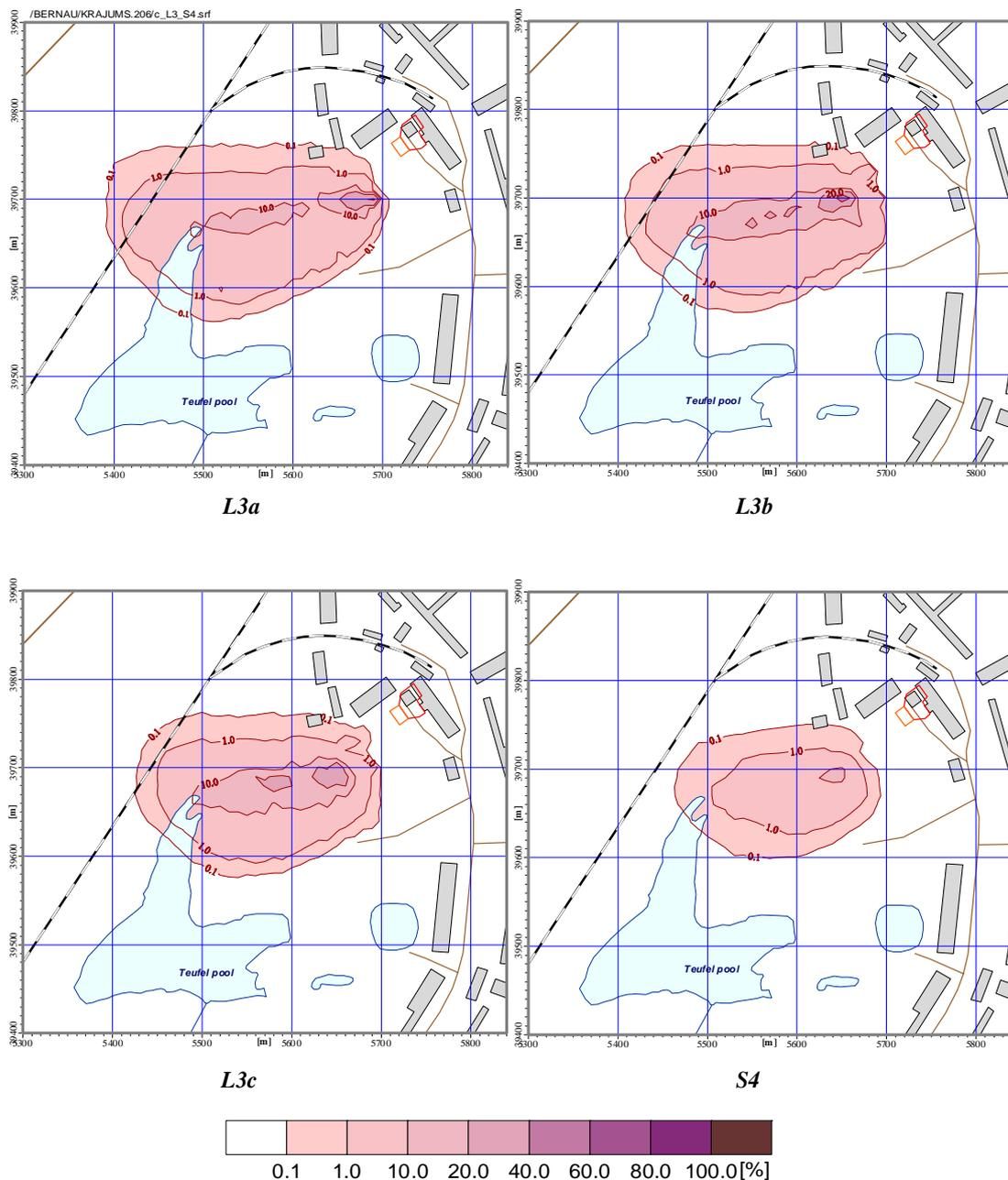
Fig 3. The first TCE source. Elapsed time 5000 days. Modelled TCE concentrations [mg/l] for the L3a, L3b, L3c, S4 layers
