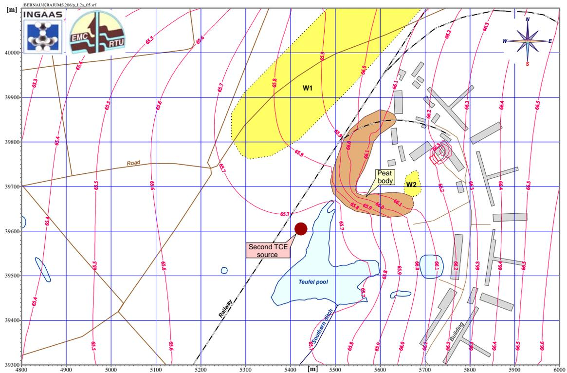
Fig 2. Corrected HM. Computed head [m asl] for the L2 aquifer; W1, W2 windows of the S2 aquitard
