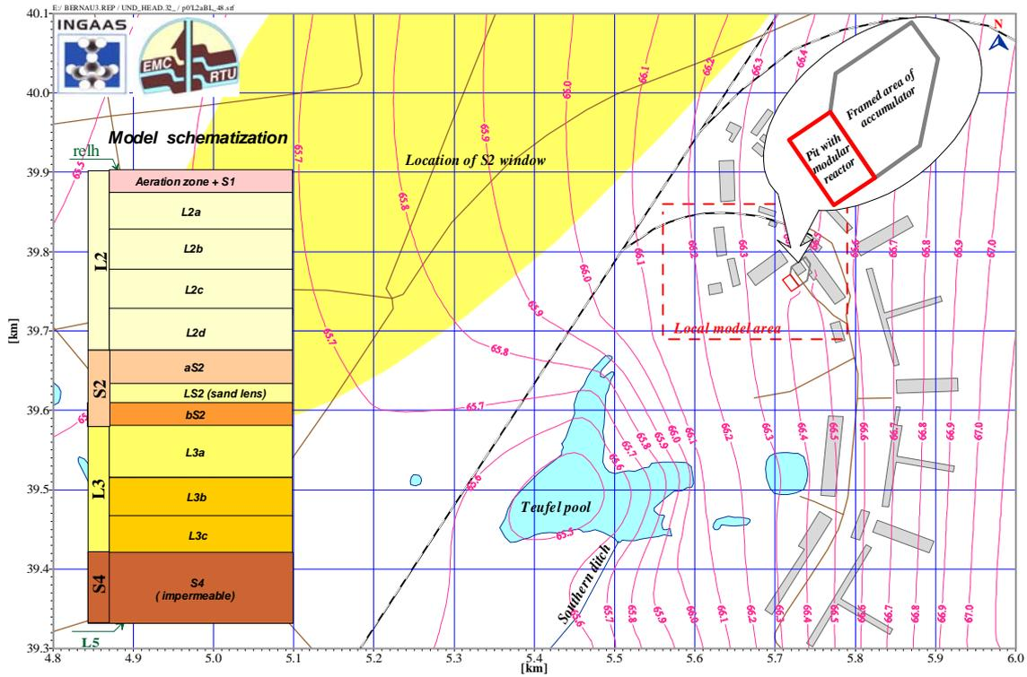
Fig 1: Original HM. Computed head [m asl] for the L2 aquifer. Model schematization. The system of accumulator - reactor
