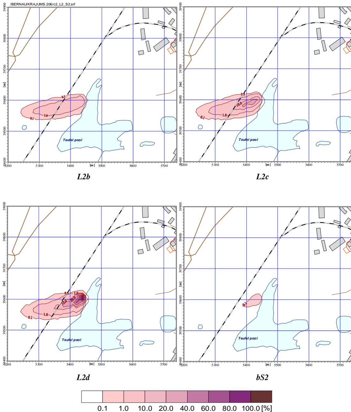
**Fig 4.** The water level of the Teufel pool is 0.3m higher than the average level. The second TCE source. Elapsed time 5000 days. Modelled TCE concentrations [mg/l] for the *L2b*, *L2c*, *L2d*, *bs2* layers
