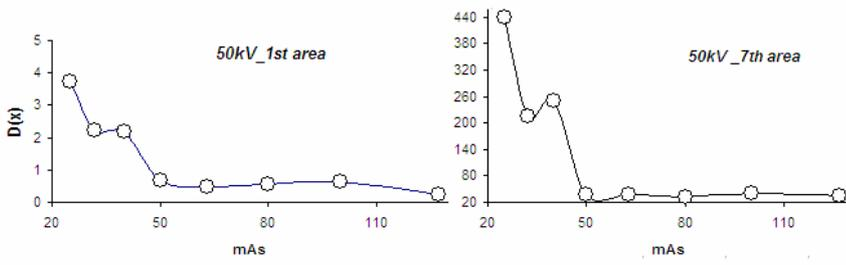
Fig. 3.  $D(x)$  of brightness histograms at 50 kV
