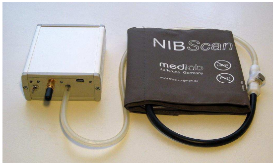
Fig. 3. System hardware. Wireless NIBP monitor
