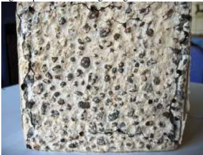
Fig. 4. Specimens of the lightweight concrete with dolomite sand after 25 frost cycles
