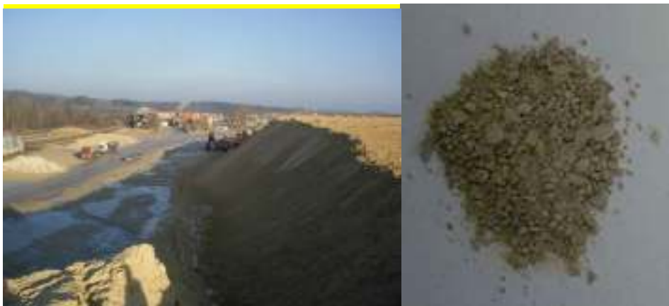
Fig. 1. Dolomit quarry (on left) and sand obtained from dolomite by-product and traditional sand (on right)
