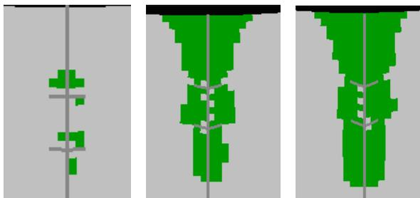
Fig 11. Shear strain development of the soil massive during the loading process
