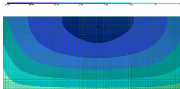
Fig 9. Deformations of the soil massive and the helical screw pile in a vertical direction
