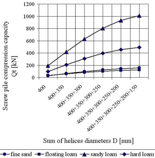
Fig 7. Compression capacity of screw piles with different number of helices.
