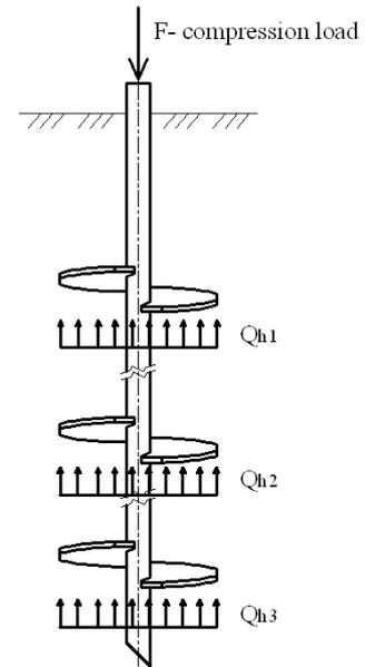
Fig 4. Design scheme of screw pile according to USA „A.B.CHANCE” company's method
