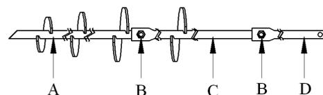
**Fig 1.** Typical configuration for a multi helix screw pile. A– lead section with several helices; B- joint; C– extension with one helix; D– extension without helices
