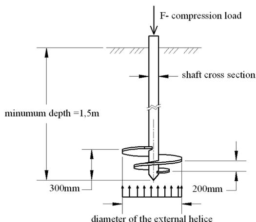
Fig 2. Design scheme of screw pile according to LBN 214-03
