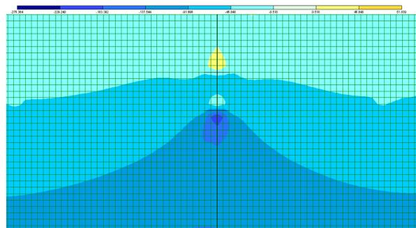
Fig 12. Soil stresses around helices
