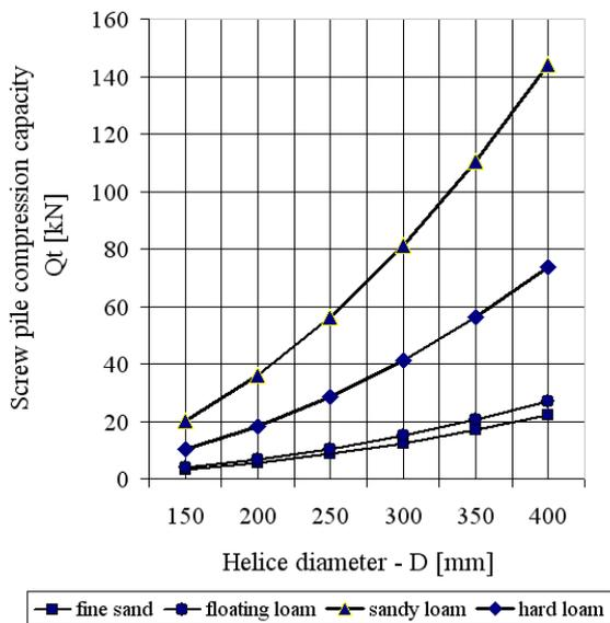
**Fig 5.** The compression capacity of screw pile in different soils depending on variety of plates diameter D, if all sizes of plates are into 150 cm depth from the top layer of soil.
