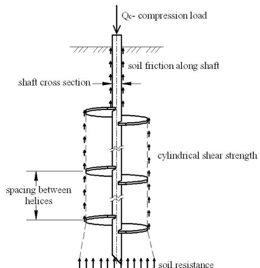
Fig 3. Design scheme of screw pile according to large capacity screw pile's method
