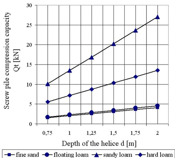
**Fig 6.** The compression capacity of a screw pile in relation to the helice depth
