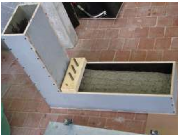
Fig. 6 L-box test (mix SCC1)
