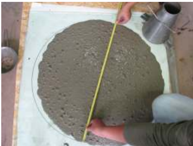
Fig. 5 Cone flow test (mix SCC2)
