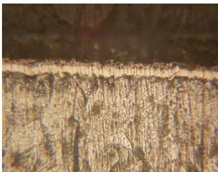
Fig.4. Microphotography of the obtained composite coating (x550)
