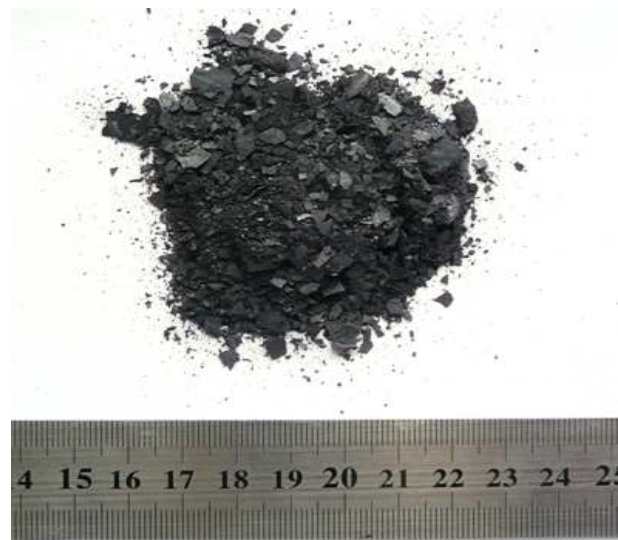
Fig. 2. Sample of iron dross
