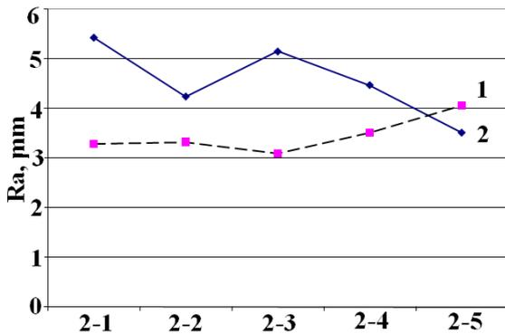
Figure 3. Ra result comparison: 1- for cutting edge angle 60 °; 2- for cutting edge angle 90 °
