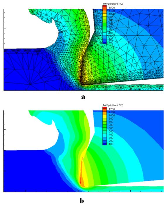
Figure 7. Simulation result of cutting process: temperature field in the cutting tool and material with meshing (a), without meshing (b)
