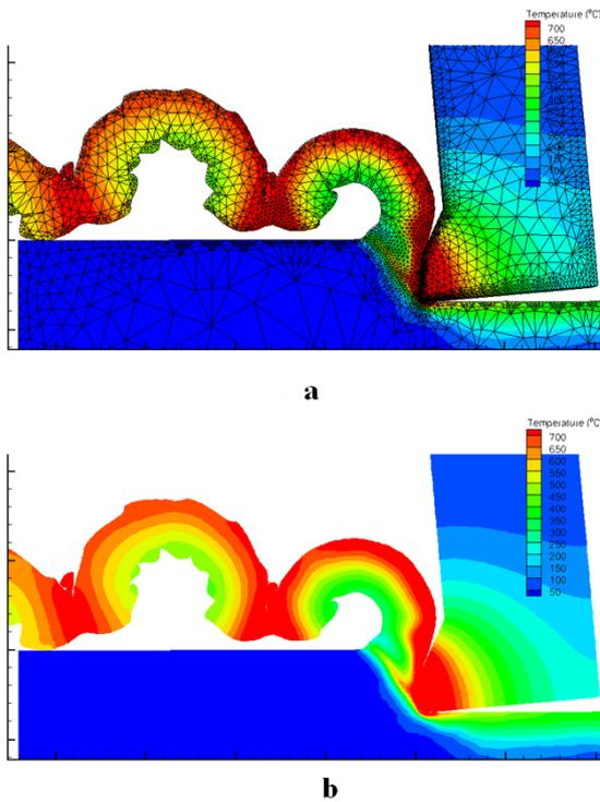
Figure 5. Simulation of cutting process, chip formation process, temperature field in the cutting tool and material distribution
