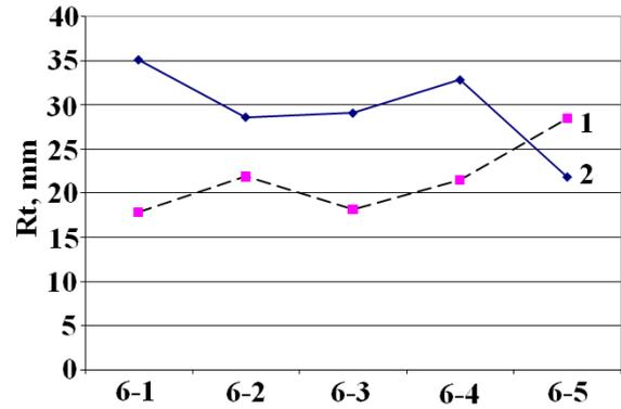
Figure 4. Rt result comparison: 1- for cutting edge angle 60 °; 2- for cutting edge angle 90 °
