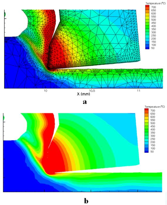
Figure 6. Simulation result of cutting process: temperature field in the cutting tool and material with meshing (a), without meshing (b)
