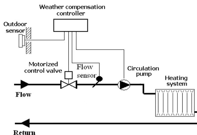
Fig. 1. Principal scheme of heating substation
