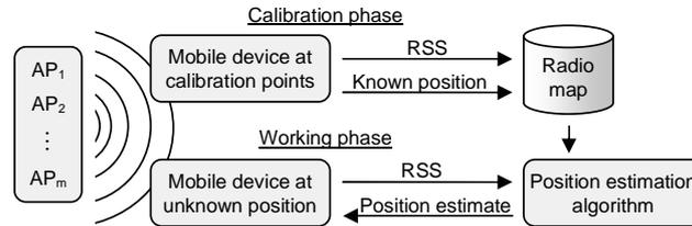
Figure 1. The two phases of location fingerprinting
