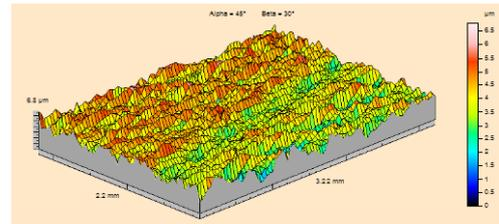
Fig .1. Surface roughness of new rotor
