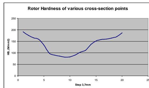
Fig.6. Change of rotor hardness
