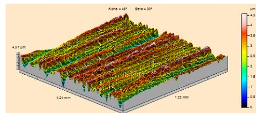
Fig.2. Surface roughness of worn out rotor
