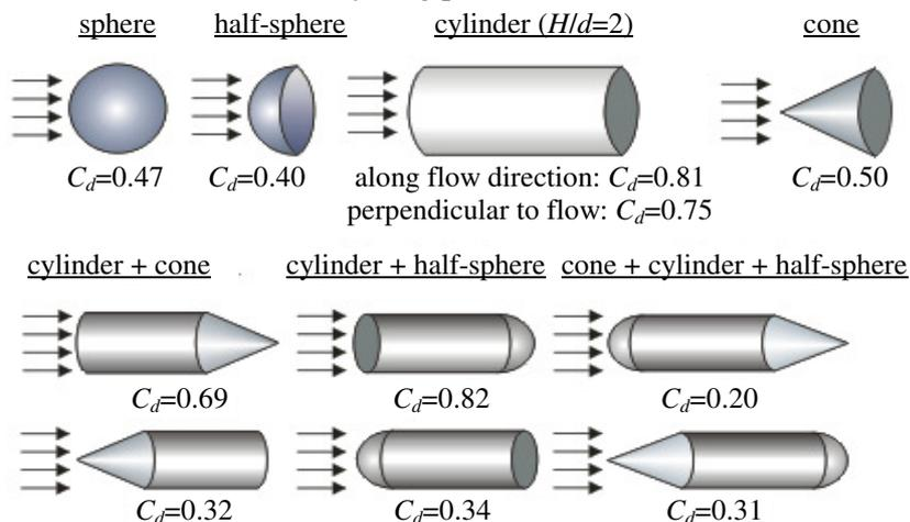
Fig. 12. Experimentally determined drag coefficients for several basic shapes
