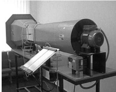
Fig. 11. Armfield wind tunnel
