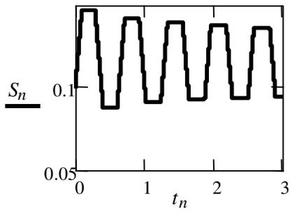
Fig. 5. Surface change in time domain taking into account bounds of switching velocity and surface limits
