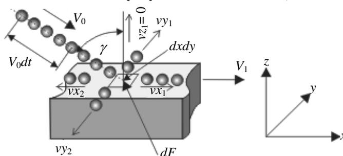
Fig. 10. Finding a force acting on a solid body in general case
