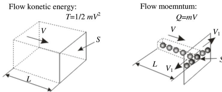
Fig. 9. Two approaches to determine force acting on plane
