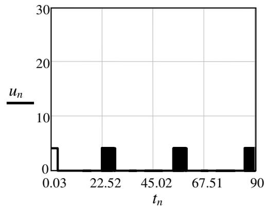
Fig. 13. Flat control action in time domain
