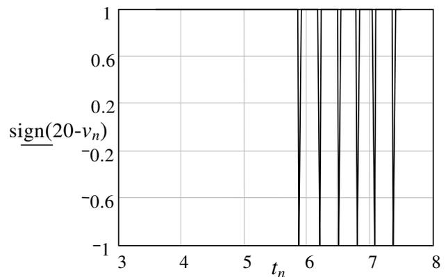
Fig. 4. “Bang-bang” control action in time region 3-8
