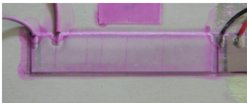
Fig.1. The cracks in piezoceramics after cyclic loading
