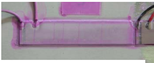
Fig.1. The cracks in piezoceramics after cyclic loading
