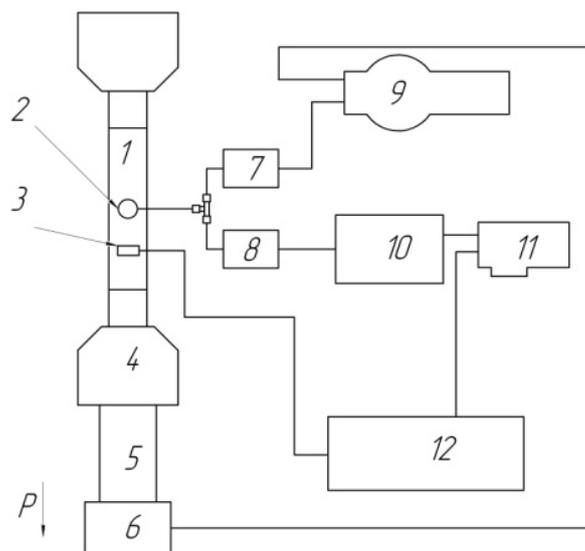
Figure 4. The scheme of switching the measuring equipment: 1 – a sample, 2 – an AE sensor, 3 a tenzogauge, 4 – a clip, 5 – a cylinder, 6 – a dynamometer, 7, 8 – preamps, 9 – PAC POCKET AE – 2, 10 – ГСП АРГУС6 7 АФ-15, 11 – LCard L-783, 12 – a strain gauge system
