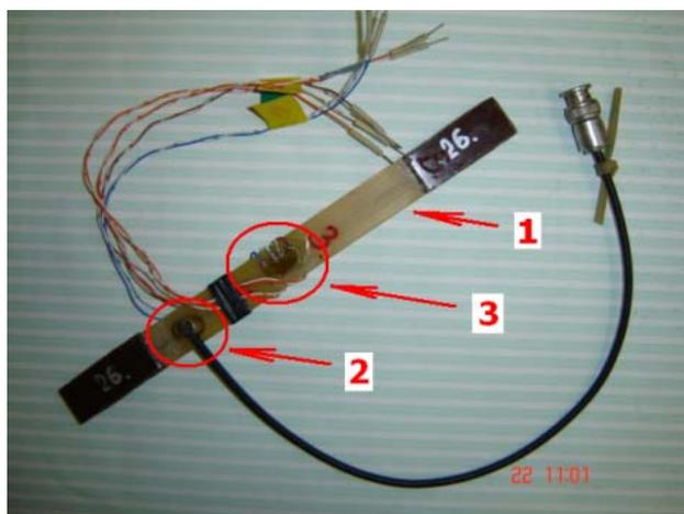
Figure 3. The attachment of the AE sensor on the sample: 1 – an AE sensor, 2 – a sample 3 – tenzogauge
