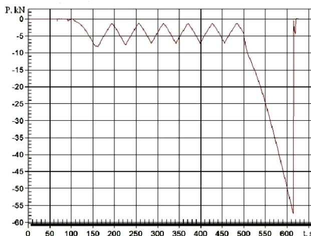
Figure 5. Schedule of sample loading with longitudinal fibres preliminary six-fold loading
