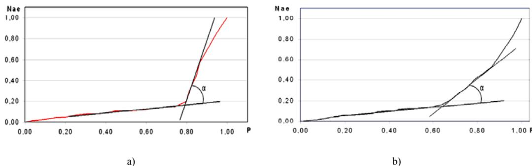
Figure 9. The graph of the relative the AE impulses summing growth versus the relative loading:
