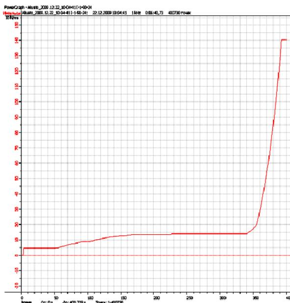
Figure 6. The total of AE signals account versus the time when the specimen was loads with a transverse arrangement of fibres with a preliminary three-times loading
