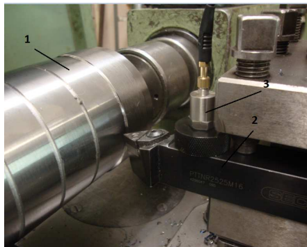
Fig. 4. Experimental test rig, 1- 420 Stainless Steel machined part, 2- cutting tool holder with the cutting insert, 3 – vibration accelerometer
