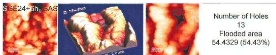
Figure 8. AFM results of the surface topography analysis of composite ceramic SGE24+6h_{ISAS}
