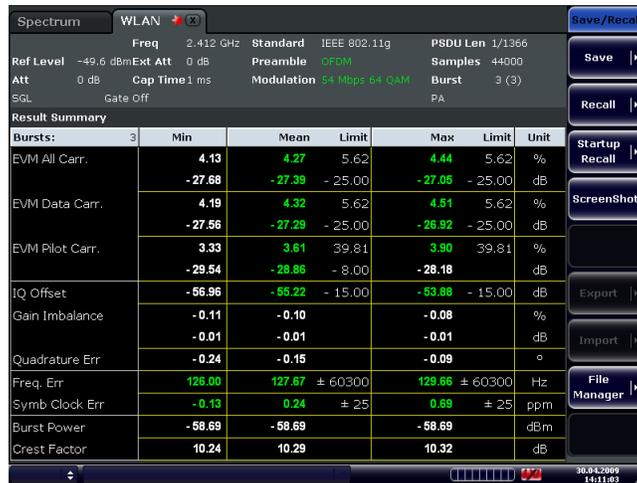
Fig. 5: EVM estimation example on the Rohde&Schwarz FSV-K91n signal analyzer
