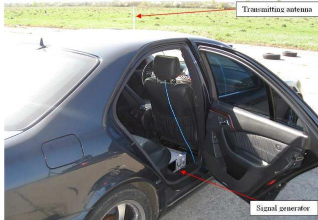
**Fig. 3:** Signal transmitting side
