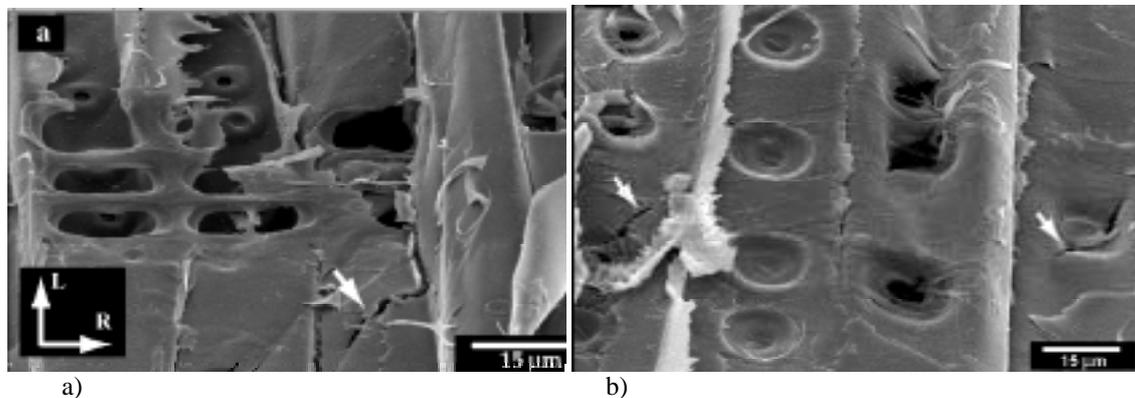
Fig. 4. Damage related to the impregnation process (marked with white arrows)
