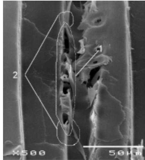
Fig. 6. Crack plane deviation initiated by cell wall damage close to the ray in case of longitudinal splitting crack in L-R plane. Damage regions: 1-weak region at the ray ends, 2-damaged cells at the ray.
