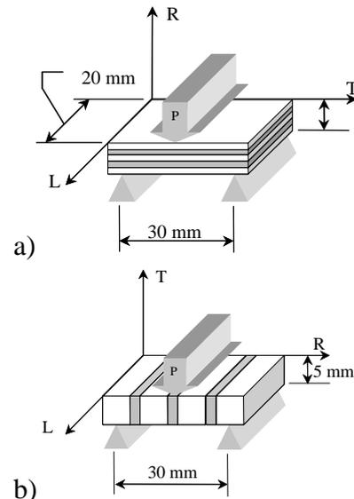
Fig.2. Scheme of 3-point flexural tests. Orientation of the specimens with respect to supports and applied load. a) T-0 test; b) T-90 test.
