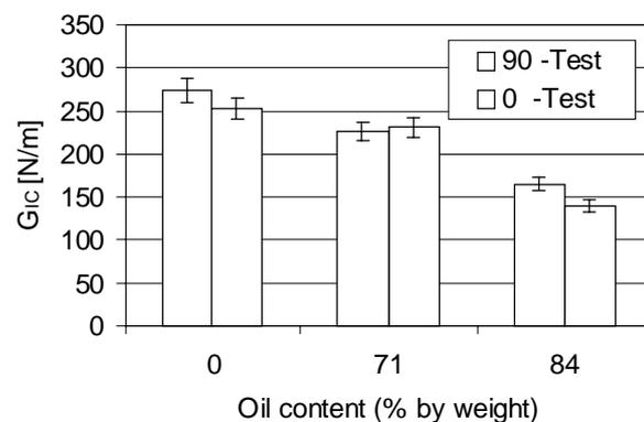
Fig. 7. Critical strain energy release rate dependence on oil content in pine, 90-test, and 0-test.
