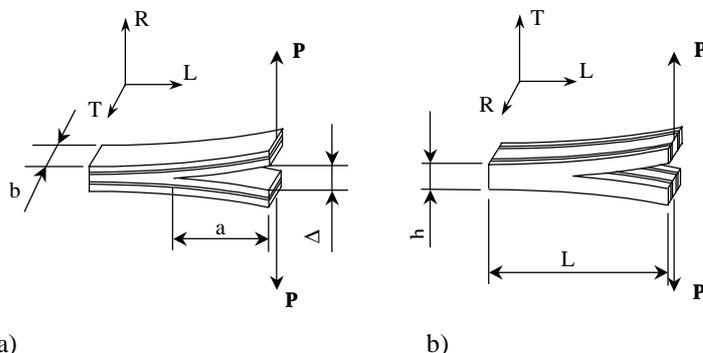
a) Fig. 1. Scheme of DCB tests specimens and loading. The annual rings are shown as a sequence of dark and white layers. a) is called 0-test b) is called 90-test.
