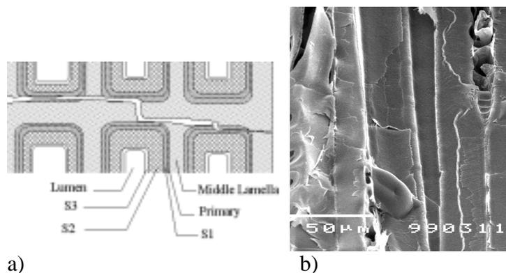
Fig. 5. Inter-cell splitting crack. a) Schematic showing of a splitting in direction transverse to wood cells, b) Splitting crack surface in L-T plane.
