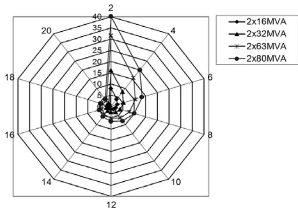
Fig. 7 Admissible TS service area  $\Pi_{TS,ij}$ , km<sup>2</sup>, from load density  $\sigma_2$ , MVA/km<sup>2</sup>, for 110/10-20 kV two-transformer substations in polar coordinates.
