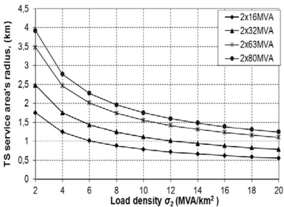
Fig. 4 Admissible TS service area's radius  $R_i$  from load density  $\sigma_2$  for 110/10-20 kV two-transformer substations.
