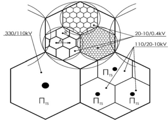
Fig. 2 The ideal model of service areas for TS of different voltage levels.
