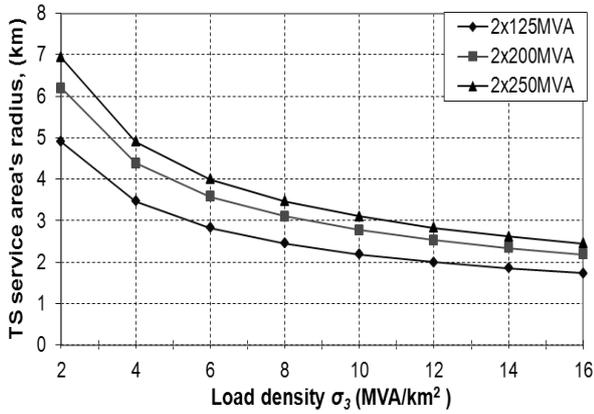
Fig. 3 Admissible TS service area's radius  $R_i$  from load density  $\sigma_3$  for 330/110 kV two-transformer substations.
