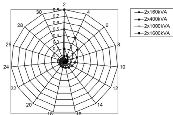
Fig. 8 Admissible TS service area  $\Pi_{TS,ij}$ , km<sup>2</sup>, from load density  $\sigma_1$ , kVA/km<sup>2</sup>, for 10-20/0.4 kV two-transformer substations in polar coordinates.
