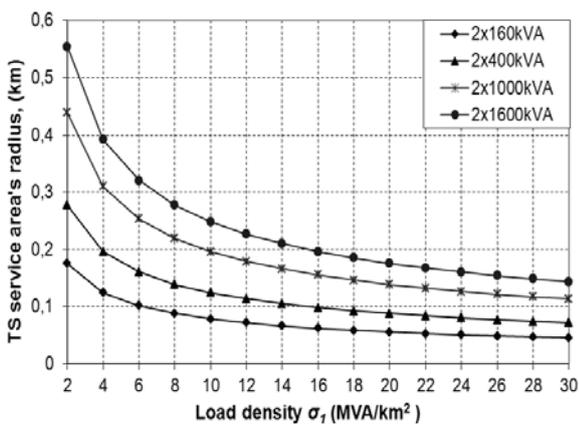
Fig. 5 Admissible TS service area's radius  $R_i$  from load density  $\sigma_1$  for 10-20/0.4 kV two-transformer substations.
