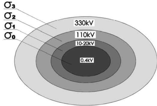
Fig. 1 UPSS hierarchy of voltage levels and load densities.
