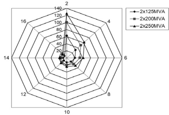
Fig. 6 Admissible TS service area  $\Pi_{TS,ij}$ , km<sup>2</sup>, from load density  $\sigma_3$ , MVA/km<sup>2</sup>, for 330/110 kV two-transformer substations in polar coordinates.
