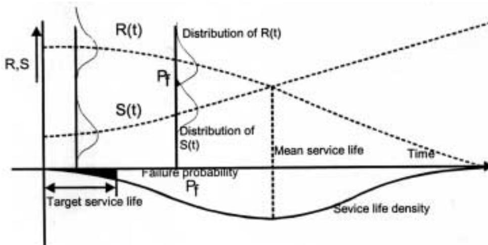
Fig. 5. Failure probability and target service life [6]
