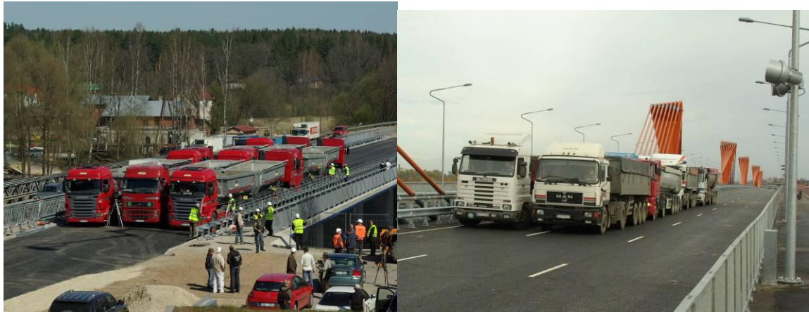
Fig.4 Static loading of Murjani and the new Dienvidu bridges
