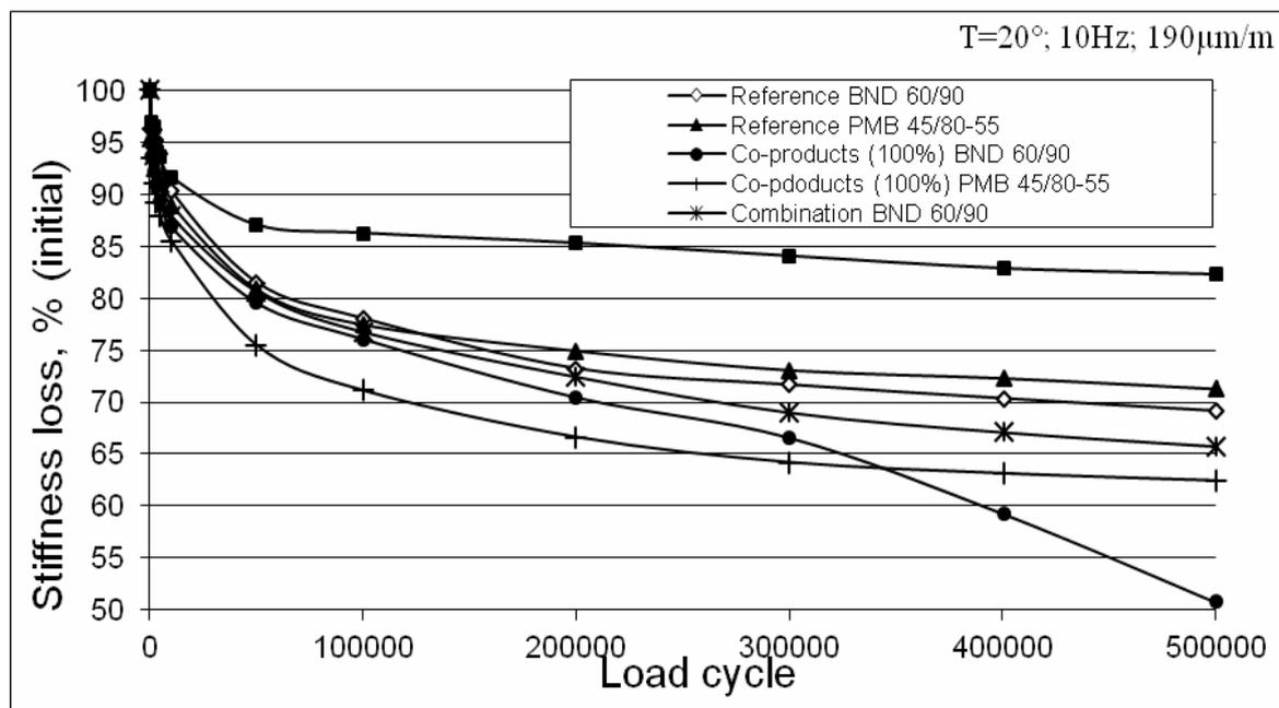
Fig. 3. Diagram of stiffness loss evolution during loading
