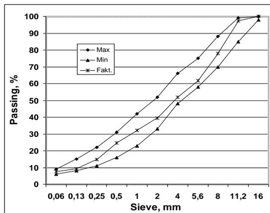
Fig. 1. Granulometry of test specimens
