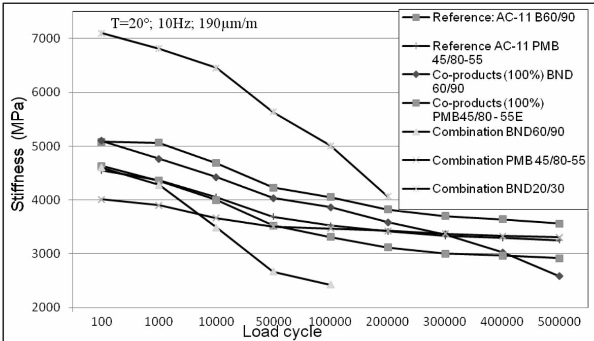
Fig. 2. Diagram of stiffness exchange during loading
