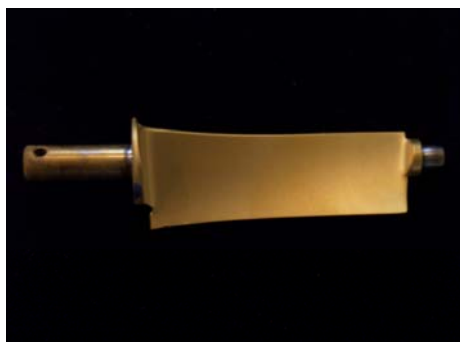
Fig.2. Stator blade of the gas-turbine engine after applying the coating
