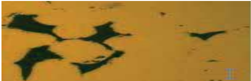
Fig. 2. Lack of fusion of separate welded layers, porosity
