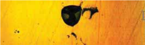
Fig. 2. Lack of fusion of separate welded layers, porosity
