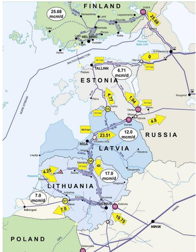
Fig.1. Maximal natural gas flow in Latvia.
