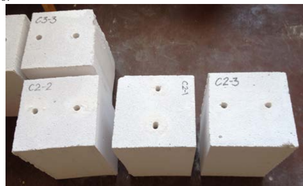
Fig.5. Aerated concrete block fragments with bores for measurement probes
