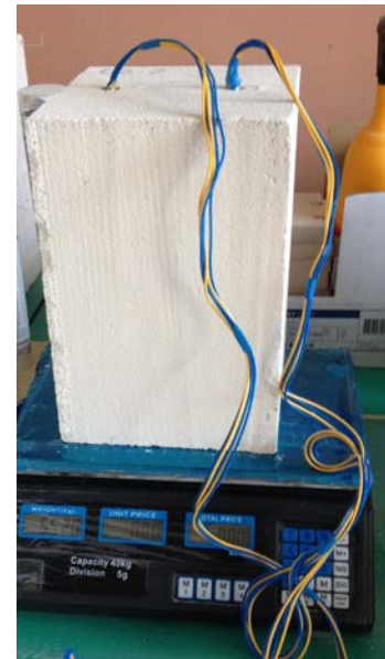
Fig.7. EIS measurements in aerated concrete block fragment (C1-1 to C3-3)
