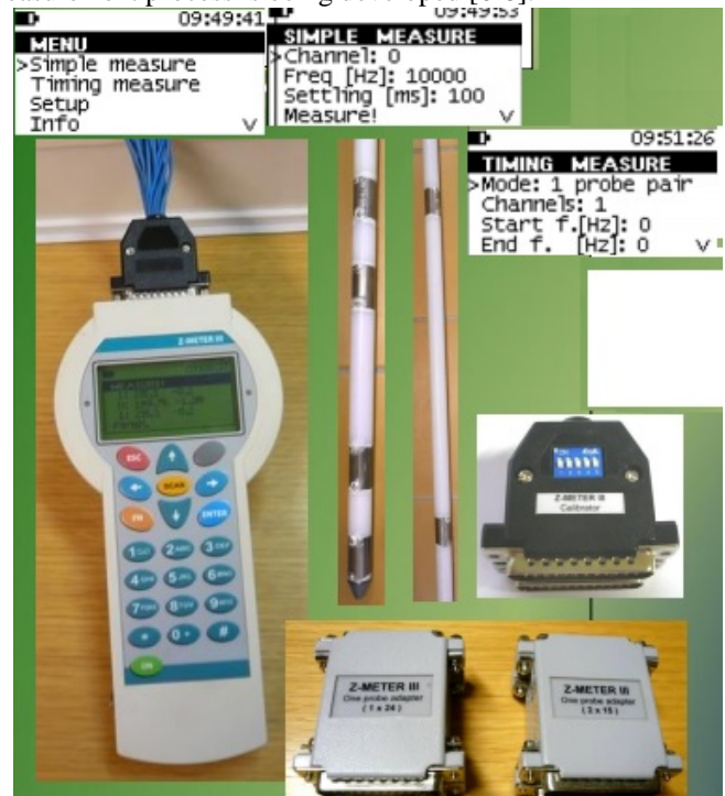
Fig.3 Z-meter III device with measurement probes and main interfaces [7]
