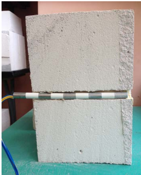
Fig.6. Example of measurement insertion in aerated concrete block fragment
