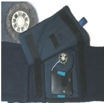
Figure 3. The prototype of the head bandage with embedded PPG device; probe contains 1 emitter and 8 detectors
