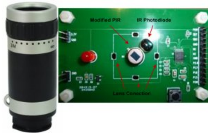
Fig. 3: Hybrid sensor board and off the shelf zoom 8X Field 9°.
