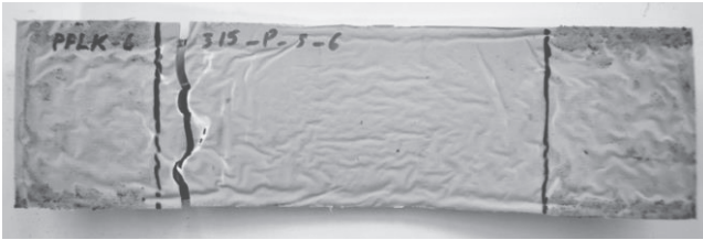
Fig.4. Obtained composite material sample breakage during the tensile strength testing
