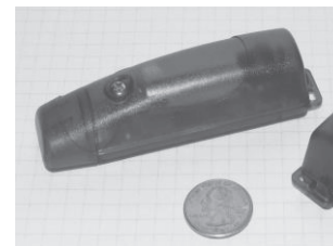
Fig. 4. Model X6-1A accelerometer ( www.gcdconcepts.com/xlr8r-1.html (accessed 1 July 2014))
